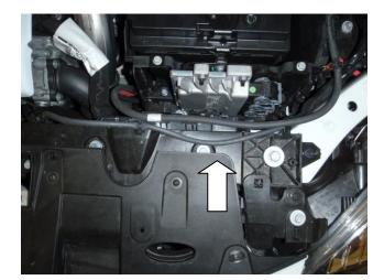
Pull the airfeed upwards to release it from the top of the bumper ,then pull the front section of the battery cover to release it from the battery
