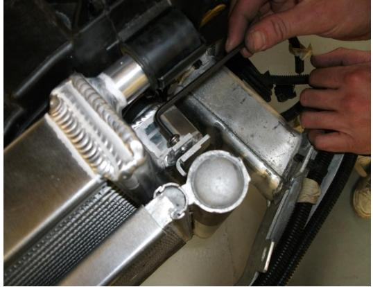
21. Undo the bleed cap on the top left hand side of radiator using a 17mm spanner .
