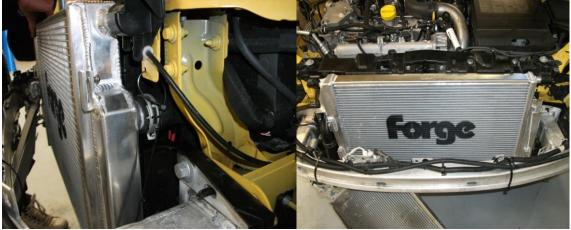
19.Now using a 10mm socket do up the left and right hand side lower bush clamps.
