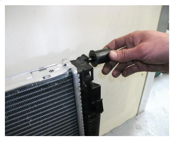
18.Once the rubber bushes are refitted to your forge radiator you can place it back into its original position, it makes it easier if you connect your inlet and outlet radiator hoses during the postioning of the radiator.
