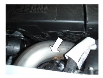
Pull the tabs out on each side of the battery cover and remove it from the car .
