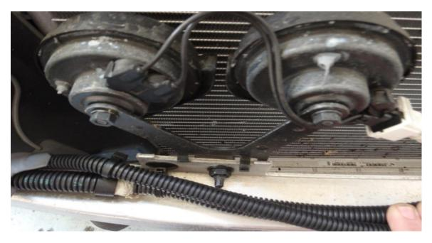
9. Use a flat headed screwdriver to prise the retaining clip out of the passenger side intercooler intercooler. When its out far enough it will 'click' into place.
