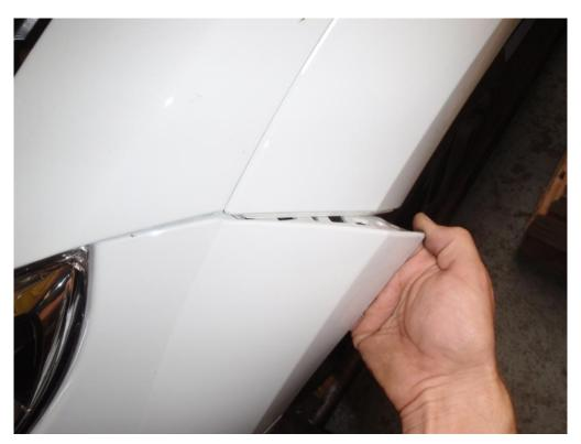
6. Lift the bumper forwards slightly off the car ,until you can access the electrical connector on the inside of the bumper passenger side (RHD)or drivers side on (LHD). Ensure the ignition is of and detach the harness
